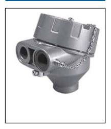
Material of body and cover : aluminium pressure die-casting, max.0.5% Mg Ambient temperature:  $T_{amb} = -40$  to  $100^{\circ}$ C - silicone rubber Coating: yellow chromating and chemically resistant paint (outside only) Maximum space for transmitter: Ø52 x 30
