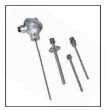
Base metal thermowell assemblies are manufactured from drilled bar stock and have threaded NPT process connections or flanges for direct immersion into high pressure or corrosive applications. Base Metal Thermocouple types are composed of common, inexpensive metals such as nickel, iron and copper. The thermocouple element can be constructed of ceramic insulated thermocouple wires or mineral insulated cable for increased durability.
