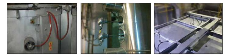
Thermocouples in Low-Pressure Die Casting
