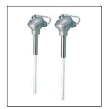
Noble Metal Thermocouples are manufactured with precious or noble metals like Platinum and Rhodium. Noble metal thermocouples can be used in oxidizing or inert applications and must be used with a ceramic protection tube surrounding the thermocouple element. Noble Metal thermocouples are designed for high temperature applications, where it is essential that the thermocouple withstands the damaging effects of oxidation and corrosion.
