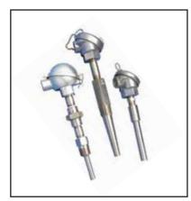
Resistance temperature detectors are designed for corrosive, high pressure, fast flowing medium with Thermowell. Resistance temperature detectors are temperature sensors that have elements which change their electrical resistance with change in temperature. RTDs with thermowell are suitable for high pressure and flow medium where there is a need for frequent change of sensor.
