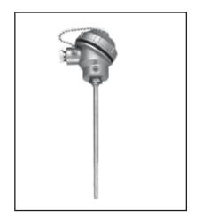
Thermocouple, complete with small aluminium enclosure (IP65 rating), 304, 316, Inconel stainless steel sheath, constructed using mineral insulated cable, ungrounded junction.
