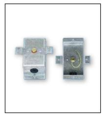
Standard Aluminum enclosure designed for all industrial and commercial surface temperature sensing applications. Fast response brass contact sensor attached to the enclosure for a low profile mating surface, Maximum temp 200°C.
