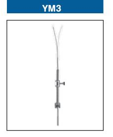
Bayonet cap type. Thermocouple complete with spring clamp and bayonet cap, constructed using thermocouple grade wires screen braided over fiber 4.8/6mm and/or screen braided over fiber glass (Round) diameter tip section, grounded junction.
