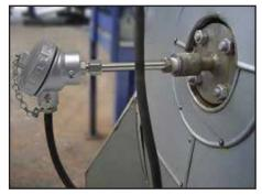
Vibration-resistant Rtd Sensor With Thermowell For Power Plant
