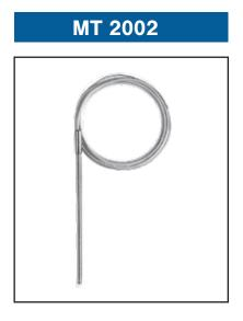
Thermocouple, complete with 2 metres PVC lead. Fiber glass, screen braided, fiber, teflon, silicone, 304, 316, Inconel stainless steel sheath, constructed using mineral insulated cable, undergrounded junction.
