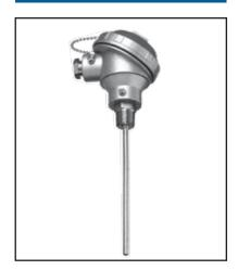
Thermocouple, complete with large aluminium enclosure (IP65 rating), 304, 316, Inconel stainless steel sheath, constructed using mineral insulated cable, ungrounded junction.
