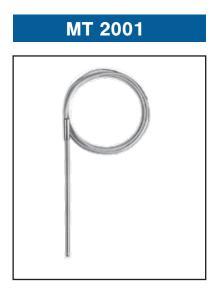
RTD 3 wire type, complete with screenfiber, silicon, PVC wire, constructed using 316 stainless steel sheath.
