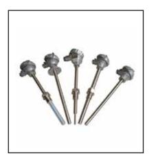
Mineral-insulated RTDs provide excellent performance, even when exposed to high levels of shock and vibration in tough industrial environments. Mineral Insulated Resistance Thermometers are made with Platinum-measuring resistors Pt100 $\Omega$  to DIN IEC 751. The measuring resistor will be connected to the inner conductors, is also embedded and is surrounded by the metal sheath to form a hermetically sealed assembly.
