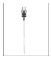
Thermocouple, complete with standard plug and tube adaptor, 304, 316, Inconel stainless steel sheath, constructed using mineral insulated cable, ungrounded junction.
