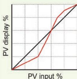
Linearisation of signals with square characteristic such as flow rate
