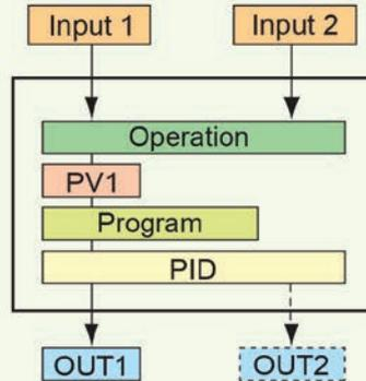
\* 2 outputs (for heating/cooling control) may also be provided.
