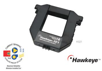
Hawkeye x21/x21SP analog current transducers provide reliable load trending information for large motor loads (up to 2400 A), with a proportional 4 to 20 mA signal. Three devices are available, each with a different amperage range. The Hx21 versions include a span potentiometer that allows each sensor to be calibrated for maximum resolution. The Hx21SP versions are factory-calibrated at a range specified by the customer.
