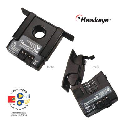
The Hawkeye Relay Combination Series combines an on/off status sensor and command relay in one package, saving the labor, wire runs, and space required to mount a separate relay. The switch and relay (not electrically connected) are in the same housing, saving space and cost. It is ideal for monitoring and controlling motors where belt loss is not a concern.
