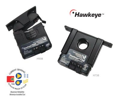
The Hawkeye Relay Combination Series is the ideal solution for the automation installer. These units combine a current switch and relay into a single package, reducing the space required for total control of fans and pumps. The current switch and relay operate independently of one another. These devices allow start/stop control and status monitoring with one device instead of two.
