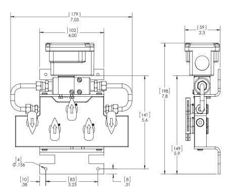
For differential pressure measurements at high line pressure (350 PSIG max), it is recommended that the pressure sensor be installed with a valve in each line, plus a shunt valve across the high and low (reference) pressure ports as shown.
