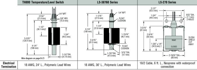
†L,= Switch actuation level, nominal (based on a liquid specific gravity of 1.0).
