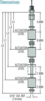
Switch actuation levels are determined following the guidelines below.
