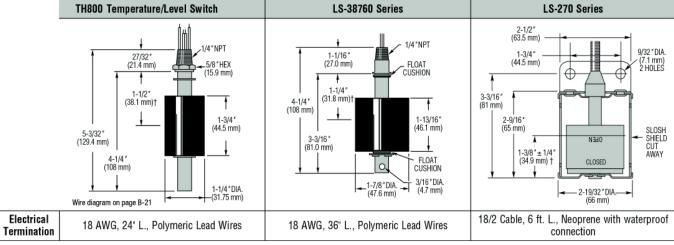
†L,= Switch actuation level, nominal (based on a liquid specific gravity of 1.0).
