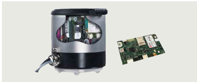
IloT Wireless Communication Module
