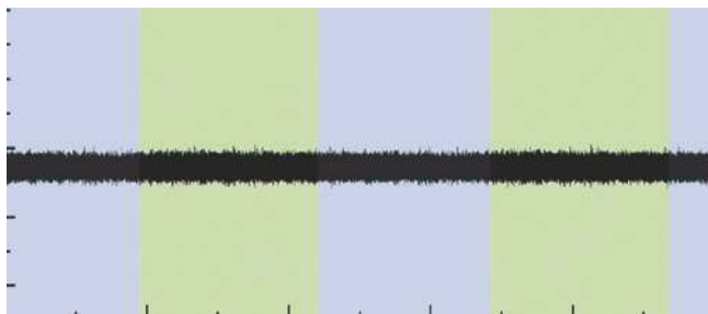
Signal from structure-borne sound sensor with intact valve
