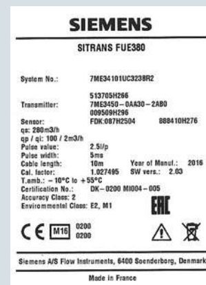
FUE380 transmitter label (with MID first verification)
