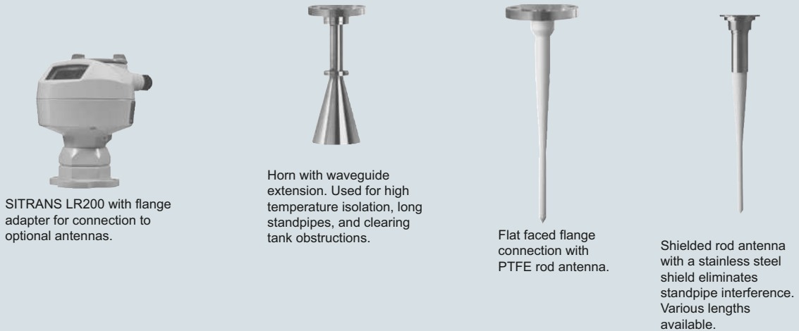
Antenna configurations for SITRANS LR200
