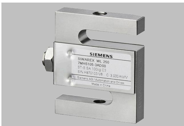
The load cell is ideal for use in tank weighing, hybrid weighing machines or suspended container weighing. It is made of stainless steel and therefore also suitable for use in harsh environments. The SIWAREX WL250 ST-S SA is suitable for both s-type tension and compression loads. The preferred direction of measurement is tension, with factory calibration for the load cells. For compression applications, adherence to the characteristic values and error limits cannot be guaranteed.
