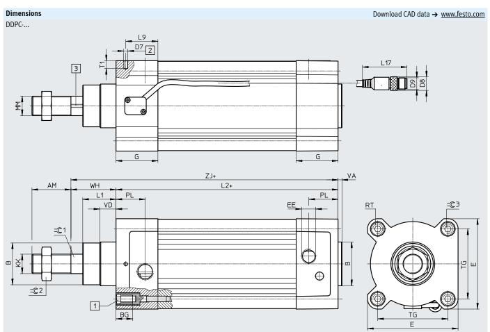
[1] Socket head screw with female thread for mounting attachments
