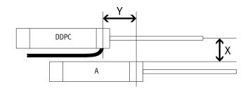
Off-set mounting, cable outlet upwards or downwards
